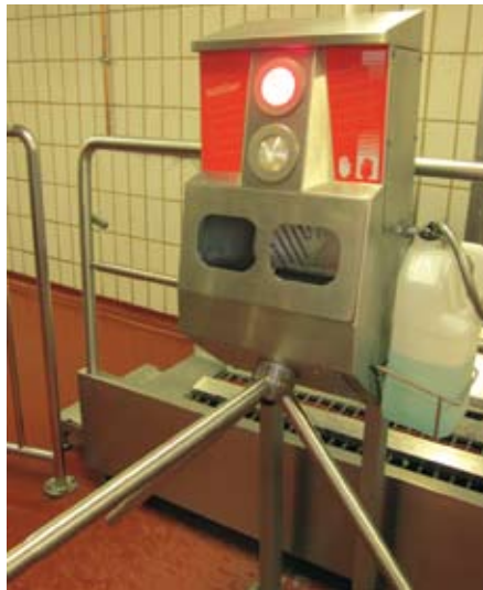
The Jwayelani Plant is HACCP compliant (accepted internationally). This is particularly important in a factory where perishable products for human consumption are handled. Stringent hygiene standards are maintained right from the time when the staff wish to enter the plant, and have soap squirted onto their hands before the turnstile will operate.
