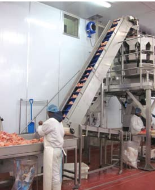
An automated multi-head weighing machine accurately portions the frozen chicken pieces and drops these into ready-branded packs for sealing.
