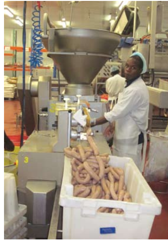
The automated sausage line currently process 2.75 tons/hour, with a capacity to process up to 8 tons/hour.
