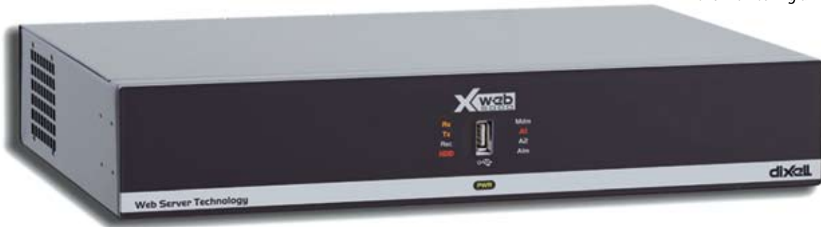
Advanced store monitoring units like this one is a specially programmed computer that monitors and computes floating suction and condensing pressures that can save around 16% of compressor power. It can also compute and send instructions for a range of other refrigeration functions such as the timing of defrosts and it can also control non-refrigeration equipment like hot water geysers.
