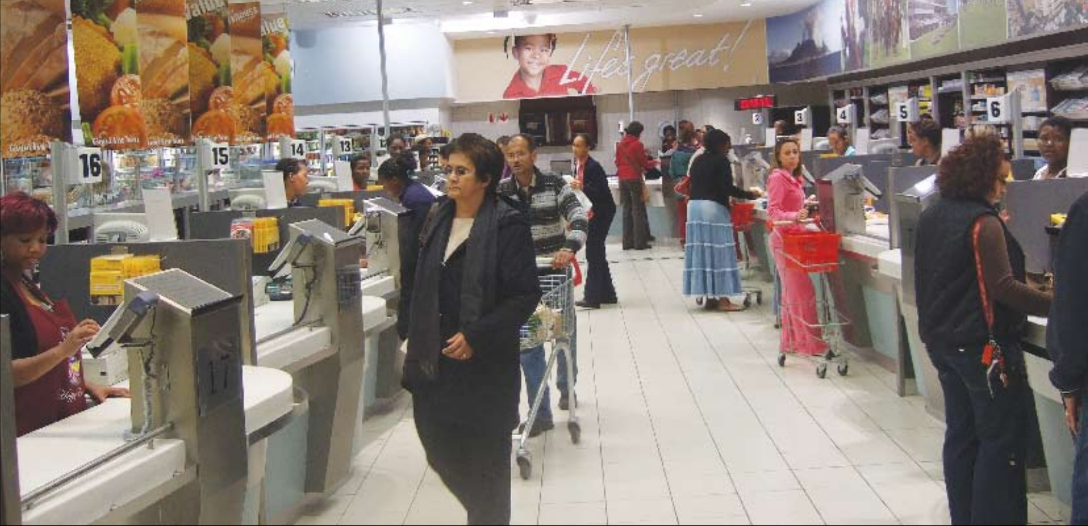
Space saving? Rosmead Superspar in Kenilworth Cape Town. This double bank system uses just half of the store front for its 16 communal queue checkouts. The right hand bank lines up against the store's front wall. The central passage effectively halves the conventional passage behind the checkouts and makes the checkout area more compact to supervise.
