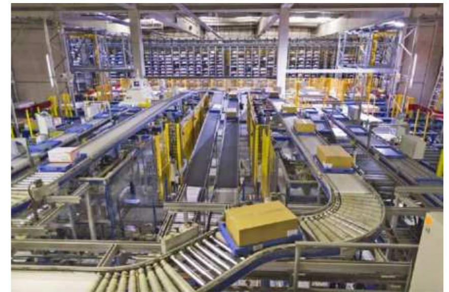
A Migros warehouse and logistics centre in Neuendorf, 2015. The automated system transports goods at -27 degrees Celsius. Keystone / Gaetan Bally
